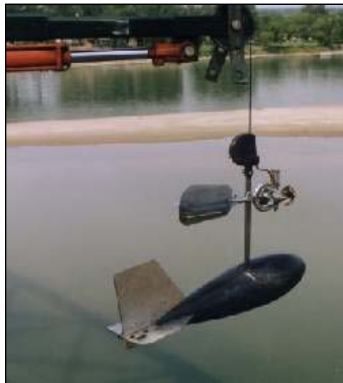
Figure 3: Example current meter used to measure water velocity.
